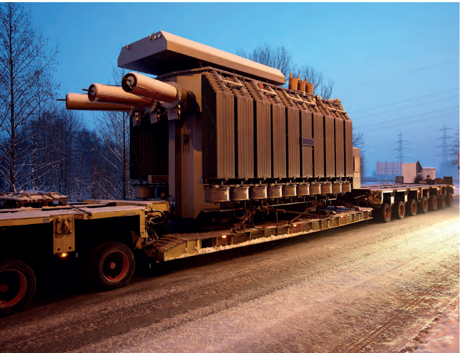
An oil-immersed transformer on its frozen way to the final place of installation. Equipped with HEROSE valves for low temperature applications.
