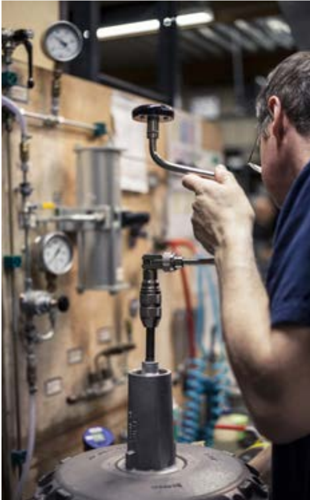
shown: brace and bit to adjust the setpoints easily
