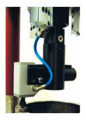
As a rule, control and reduction valves of the globe type have an integrated plug that narrowly constrains the tolerances for the seat position. In the event of damage to the seat, it is often unfeasible or extremely expensive to dismantle the valve from the pipe system in order to repair it in the workshop. If the damage is to be repaired in situ, the device to be used must be of stable construction without being bulky or heavy.
