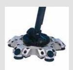
The LarsLap model G can do both gate and globe valves due to the unique flexibility of the driving unit.
