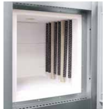
Vertically mounted SiC rods
