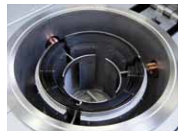
Cylindrical retort with tungsten heating
