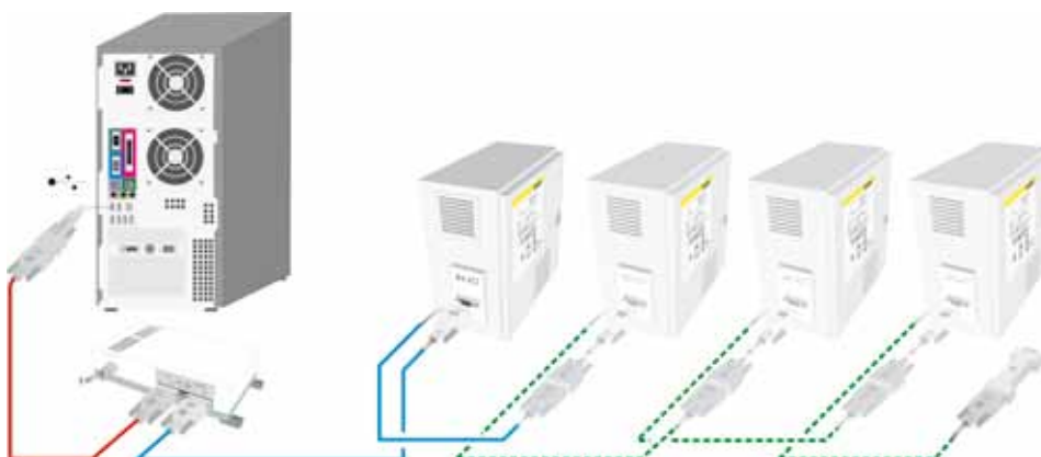
Extendable for connection of up to 16 furnaces
