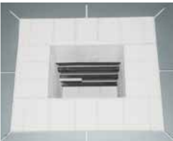
Two-Side heating with SiC rods
