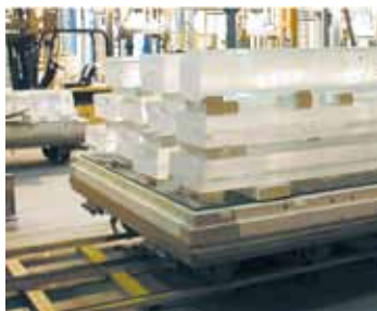
Bogie hearth furnace for tempering quartz rods
