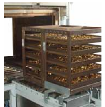
Continuous belt furnace for bulk materials in baskets
