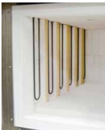
Protection of heating elements against mechanical damage
