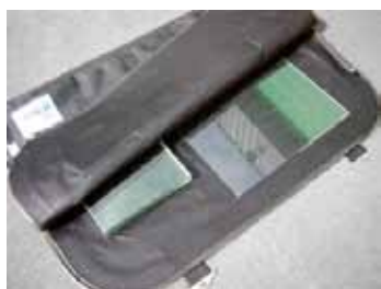
Vacuum bag for laminated safety glass
