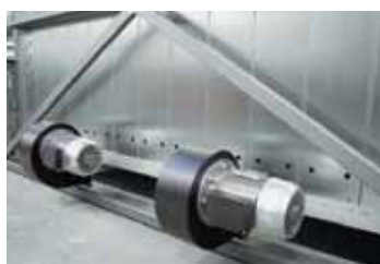
Indirect cooling behind the insulation for reduction of turbulences in the furnace chamber
